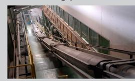
The extruded cable core is cured in a circulating inert gas environment, provides the following features.
